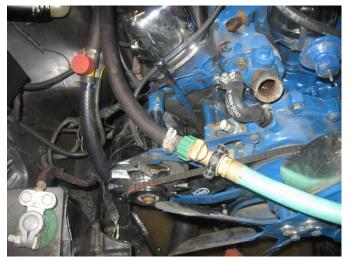
Simple procedure to get the rust and coolant buildup out of your clogged or dirty heater core.
